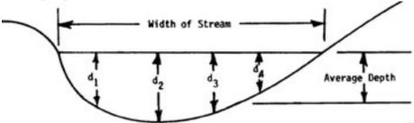
Using the diagram as a guide, use one tape measure to lay a transect across the stream. Then use the other tape to measure stream depth at a regular interval point (be sure to record the interval width (W) and have at least 5 depth measurements). Calculate the area using the following equation.
